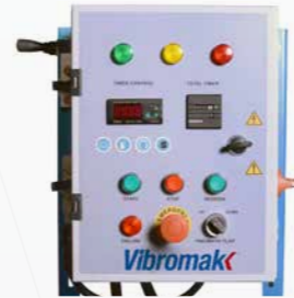
Electric Control Panel Elektrik Panosu
